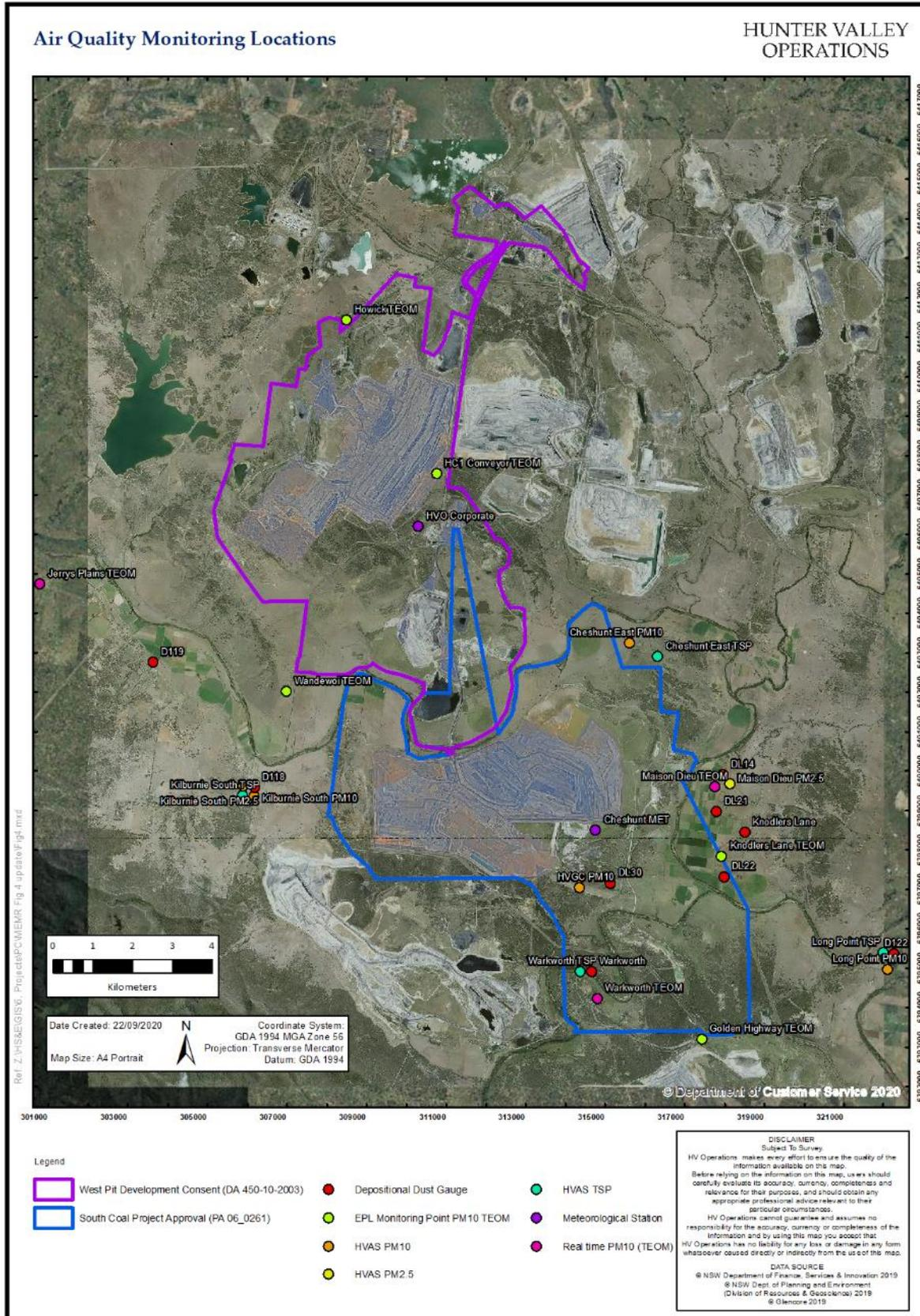
Figure 4 - Air Quality Monitoring Location Plan
