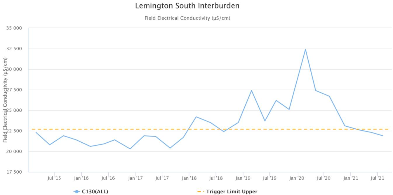
**Figure 57 - Lemington South Interburden Electrical Conductivity Trend - Q3 2021**
