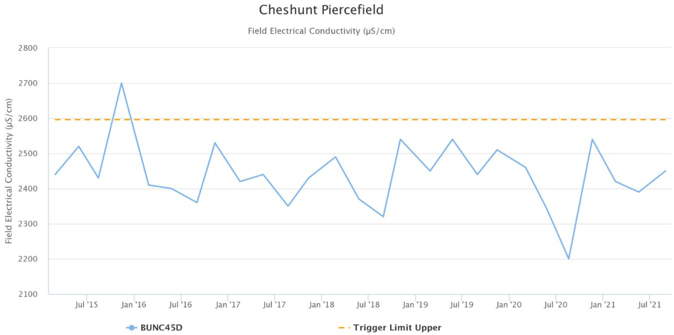
**Figure 69 - Cheshunt Piercefield Electrical Conductivity Trend - Q3 2021**
