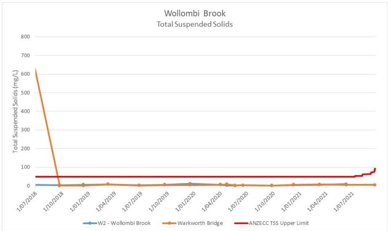
Figure 19 - Wollombi Brook Total Suspended Solids – September 2021
