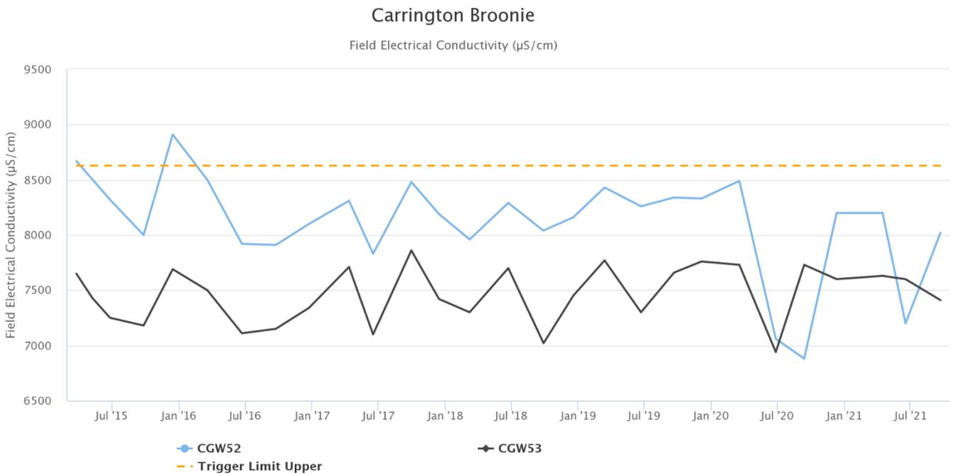
Figure 66 - Carrington Broonie Electrical Conductivity Trend - Q3 2021
