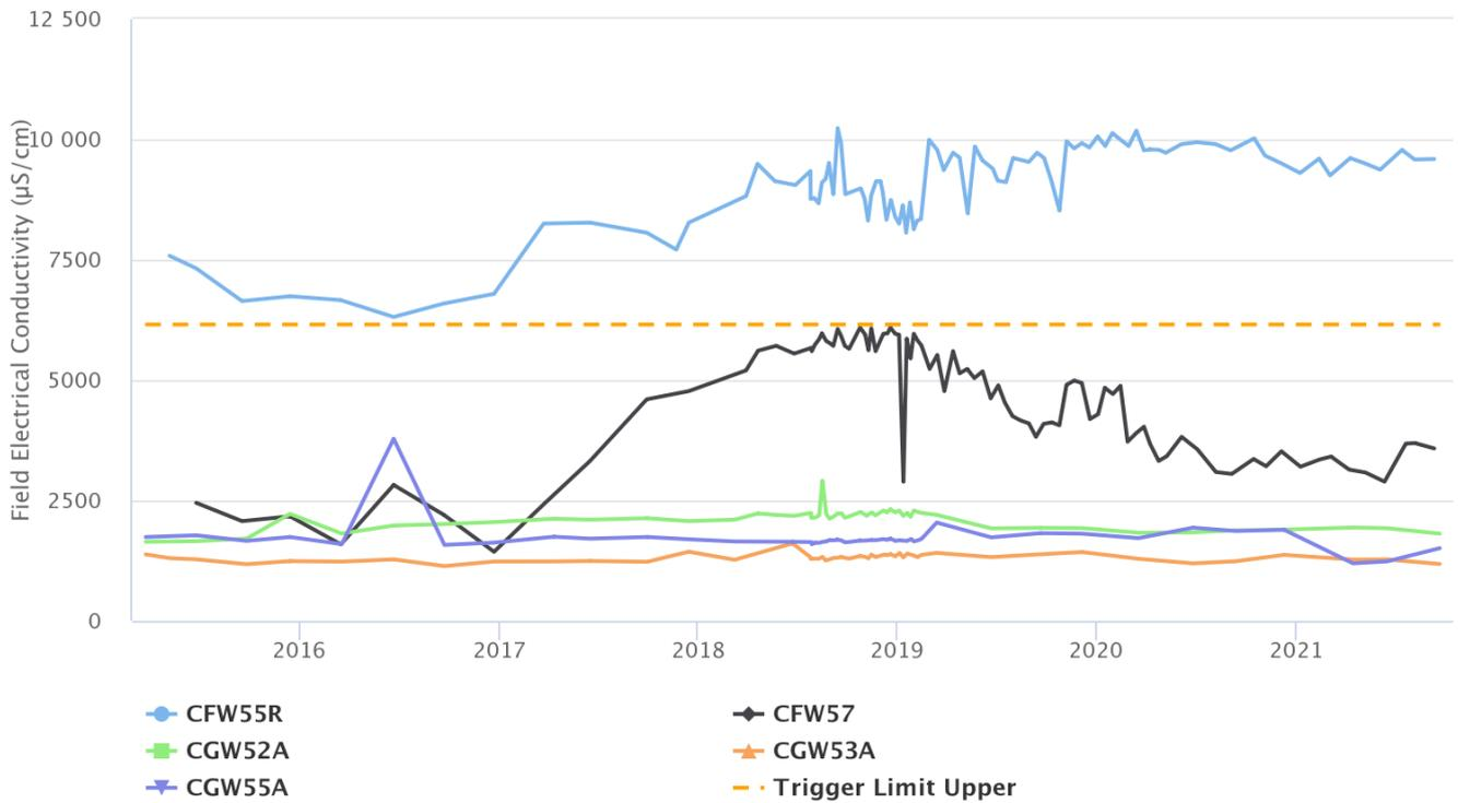
Figure 27 - Carrington Alluvium Electrical Conductivity Trend – Q3 2021
