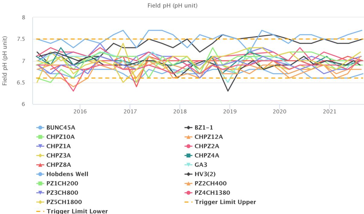
Figure 40 - Cheshunt North Pit Alluvium Field pH Trend - Q3 2021
