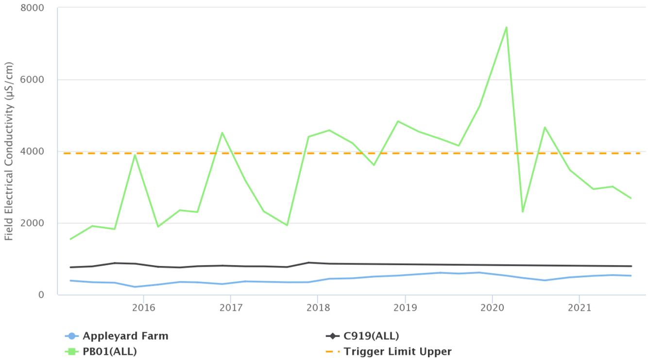
**Figure 45 - Lemington South Alluvium Electrical Conductivity Trend - Q3 2021**
