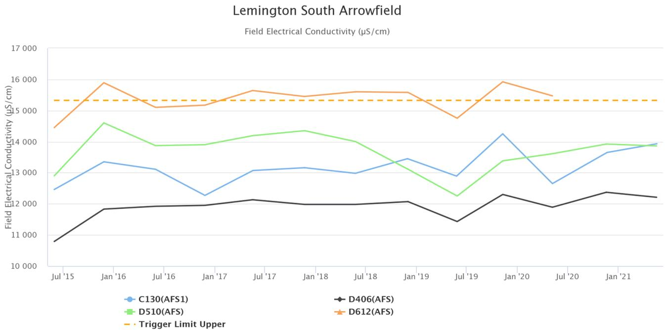
Figure 48 - Lemington South Arrowfield Electrical Conductivity Trend - Q3 2021
