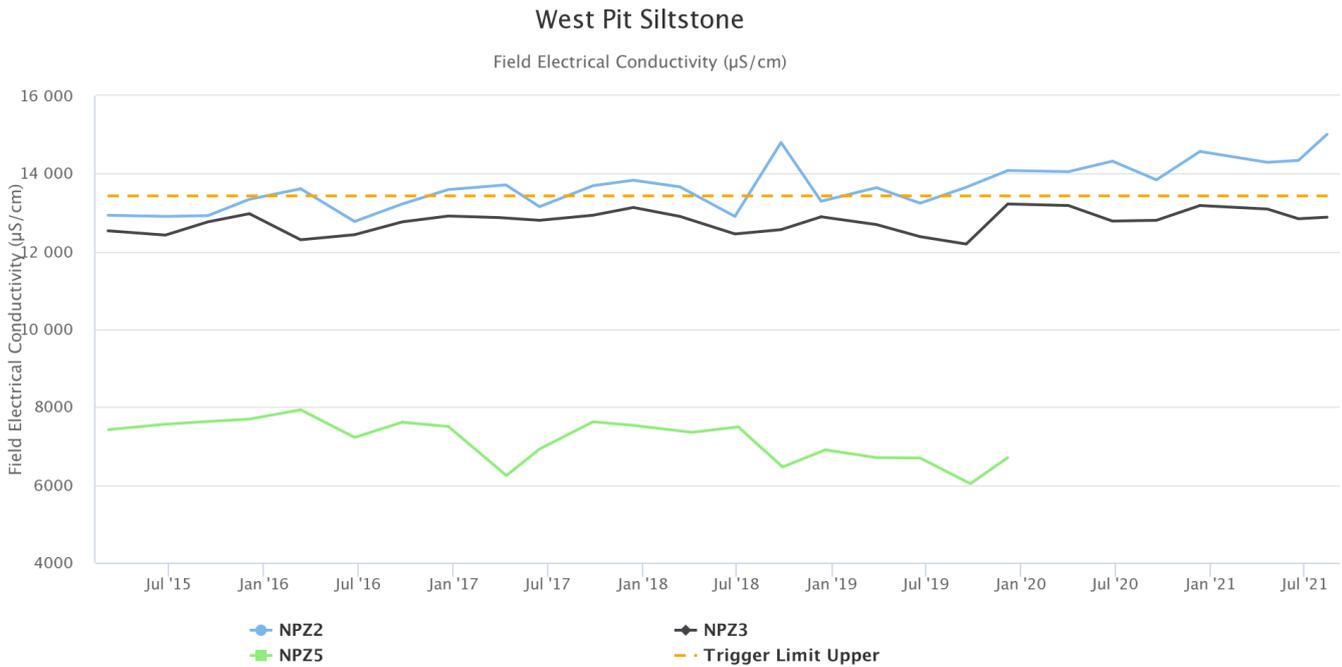
**Figure 63 - West Pit Siltstone Electrical Conductivity Trend - Q3 2021**
