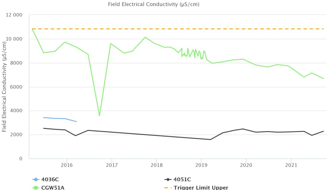
Figure 30 - Carrington Interburden Electrical Conductivity Trend - Q3 2021
