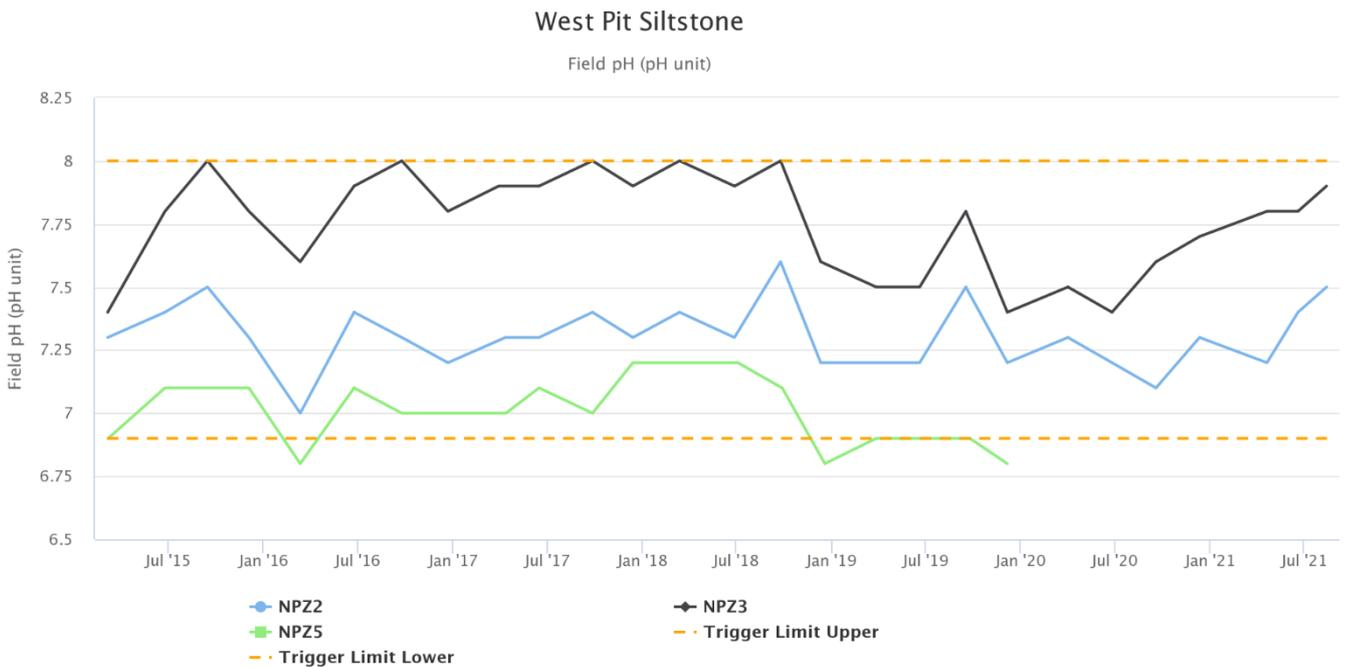
**Figure 64 - West Pit Siltstone Field pH Trend - Q3 2021**
