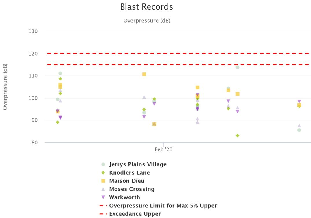
**Figure 9: Overpressure Blast Monitoring Results – February 2020**
