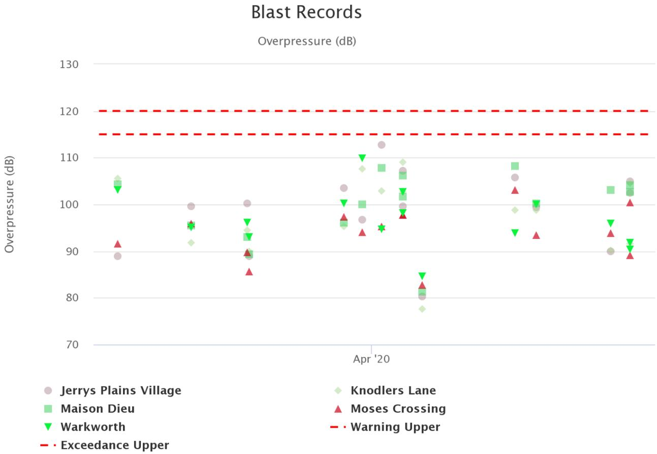
Figure 12: Overpressure Blast Monitoring Results – April 2020
