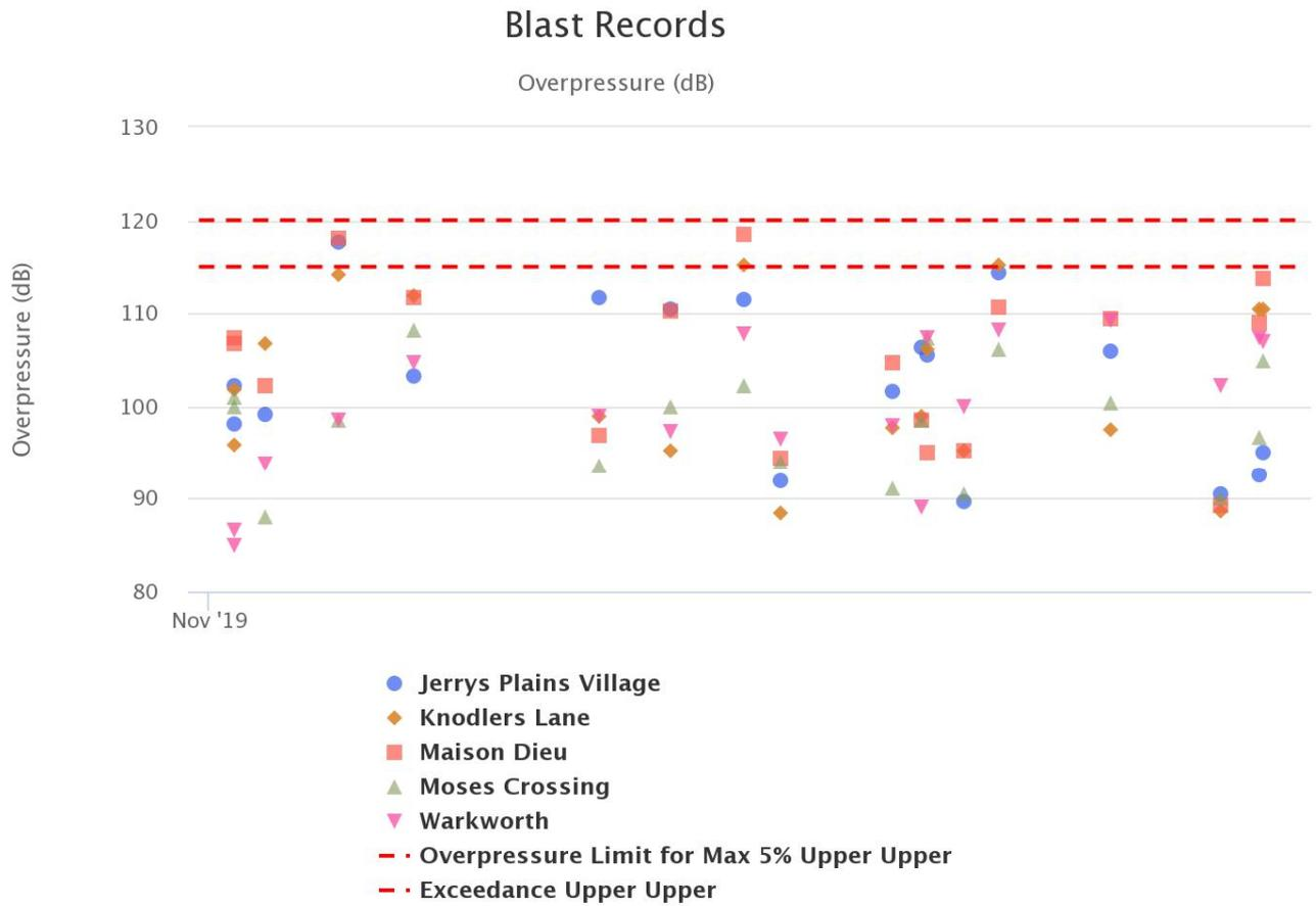
**Figure 10: Overpressure Blast Monitoring Results – November 2019**
