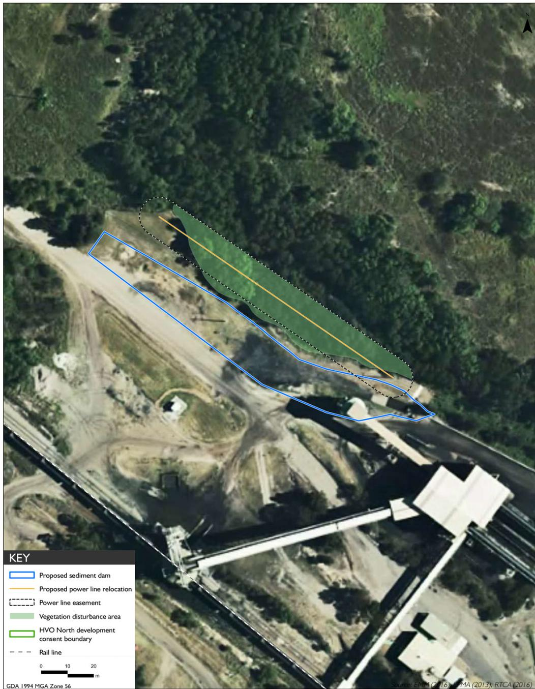
**Figure 3.1 Proposed location of the sediment basin and the relocated powerline corridor indicating the overstorey vegetation to be removed**
