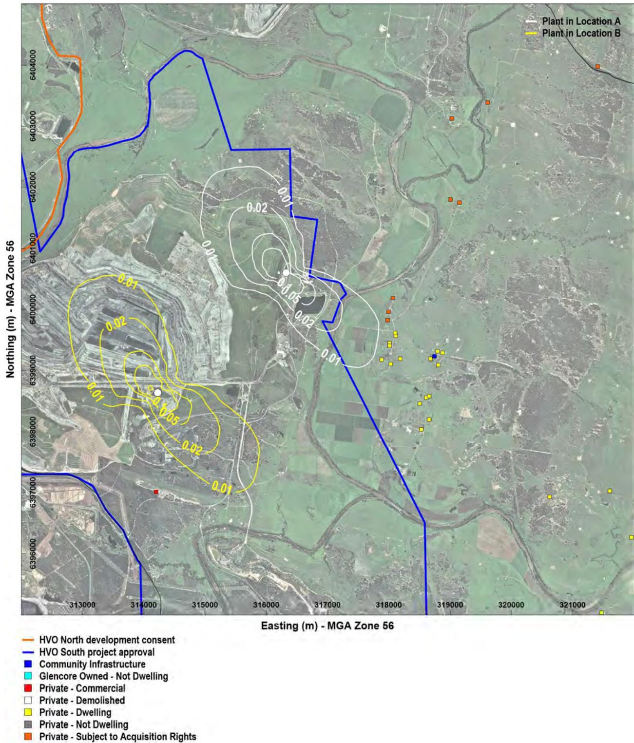
Figure B4 Predicted annual average NO<sub>x</sub> concentrations due to ANE plant (µg/m<sup>3</sup>)
