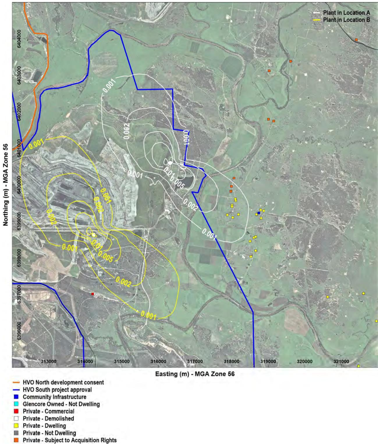
Figure B6 Predicted annual average PM<sub>10</sub> concentrations due to ANE plant (µg/m<sup>3</sup>)
