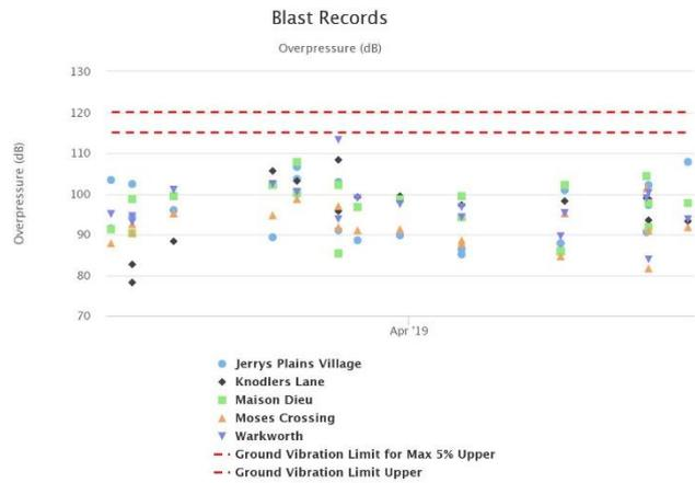
**Figure 10: Overpressure Blast Monitoring Results – April 2019**
