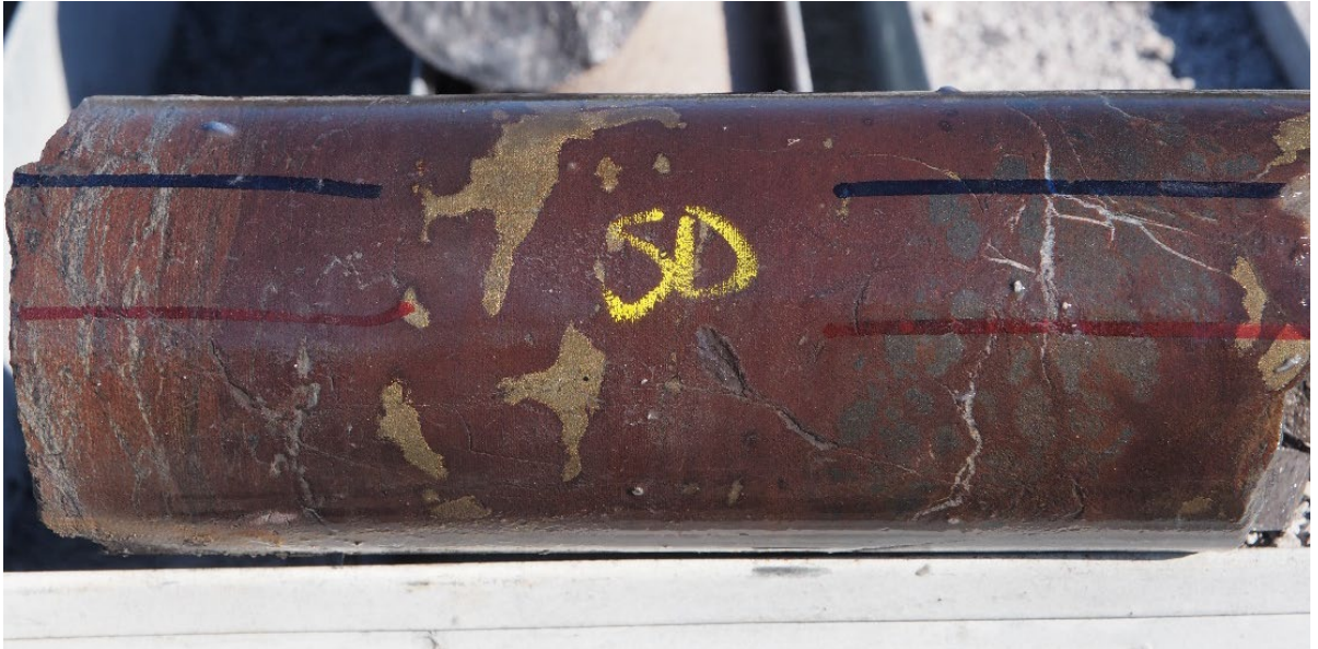
Plate 12: Siderite with pyrite blebs and calcite veinlets. Hole 4505C depth 241.8—241.95m.
