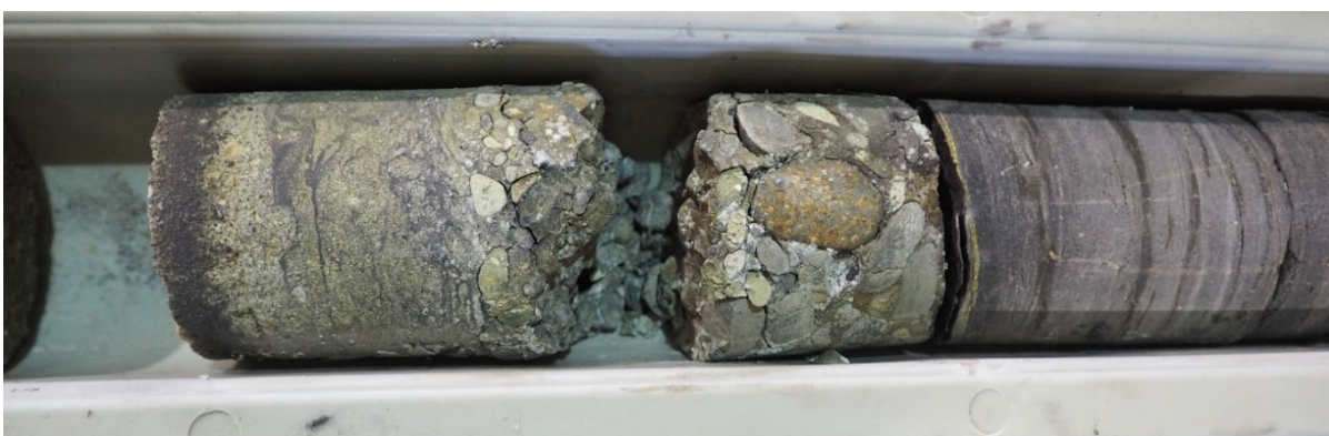
Plate 7: Iron staining and sulphate salts due to the partial oxidation of pyritic conglomerate zone above Lemington A seam. Hole 4095C depth 55.6m.
