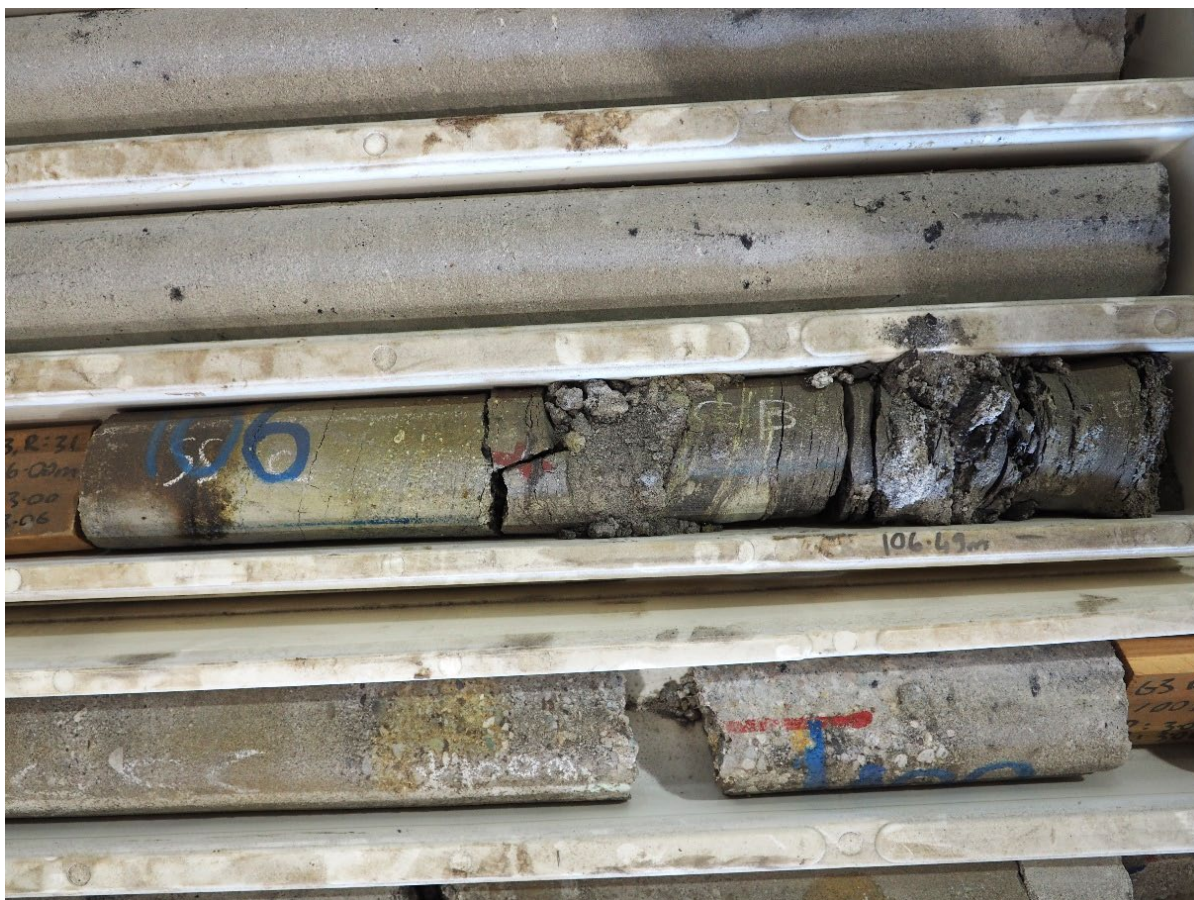
Plate 8: Pyritic zone within Archerfield Sandstone. Hole G3 depth 106m.
