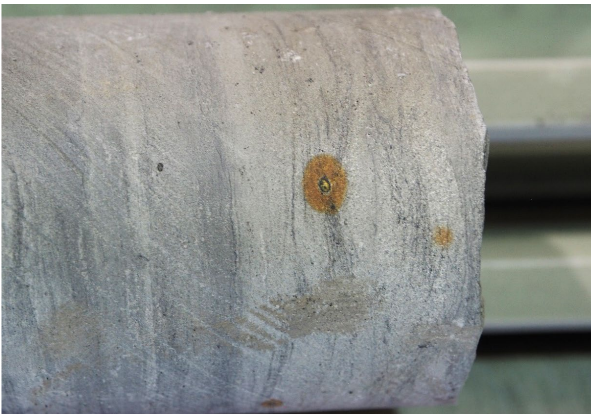
Plate 3: Iron staining and sulphate salts due to the partial oxidation of an isolated pyritic spheroid bleb in sandstone. Hole 4095C depth 57.75m.
