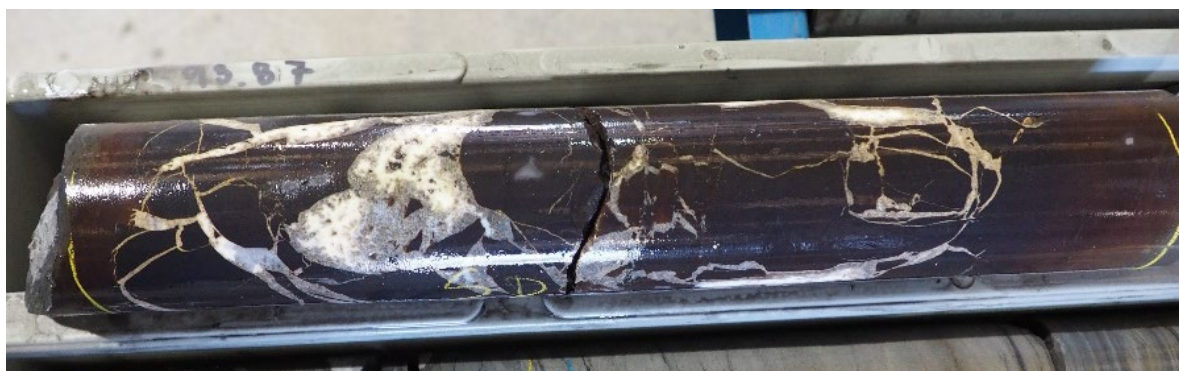
Plate 15: Siderite lens with calcitic veining and matrix. Hole 4095C 94.7m.
