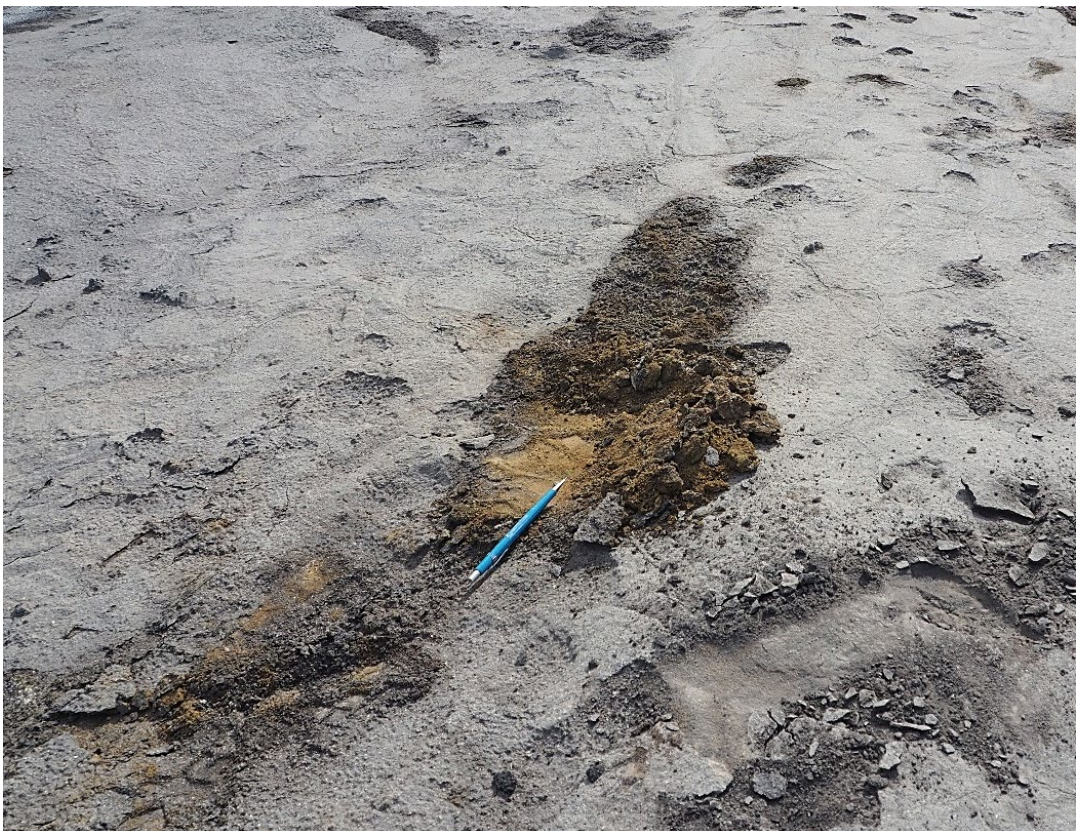
Plate 24: Iron stained pyritic materials concentrated close to spigot points within the disused Bob's Dump TSF.
