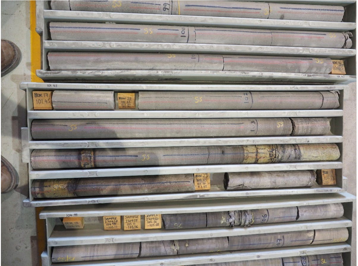
Plate 10: Generally benign Archerfield Sandstone but with pyritic zones towards its base close to Lemington A seam (removed), and pyritic zone in siltstone below Lemington A. Hole 4505C depth 99-107m.
