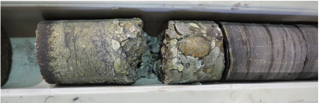
Plate 7: Iron staining and sulphate salts due to the partial oxidation of pyritic conglomerate zone above Lemington A seam. Hole 4095C depth 55.6m.
