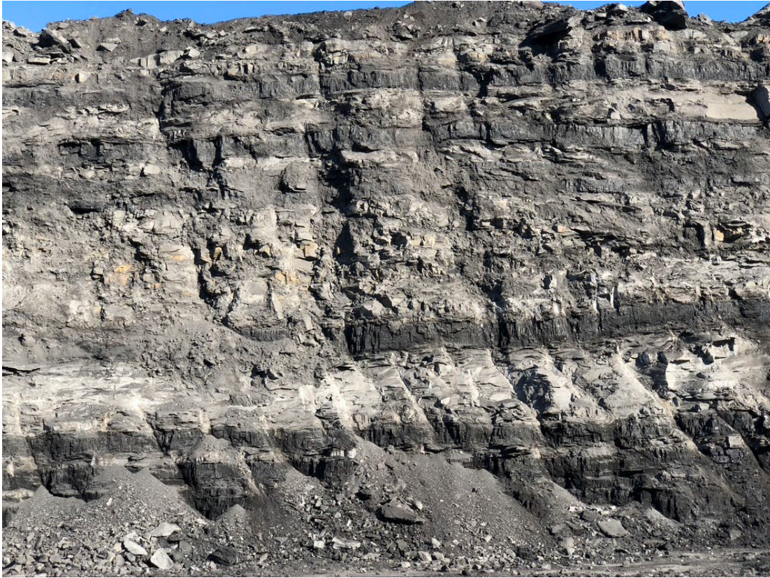
Plate 21: Cheshunt Pit 2 with iron staining and jarosite between the Piercefield and Vaux Seams.
