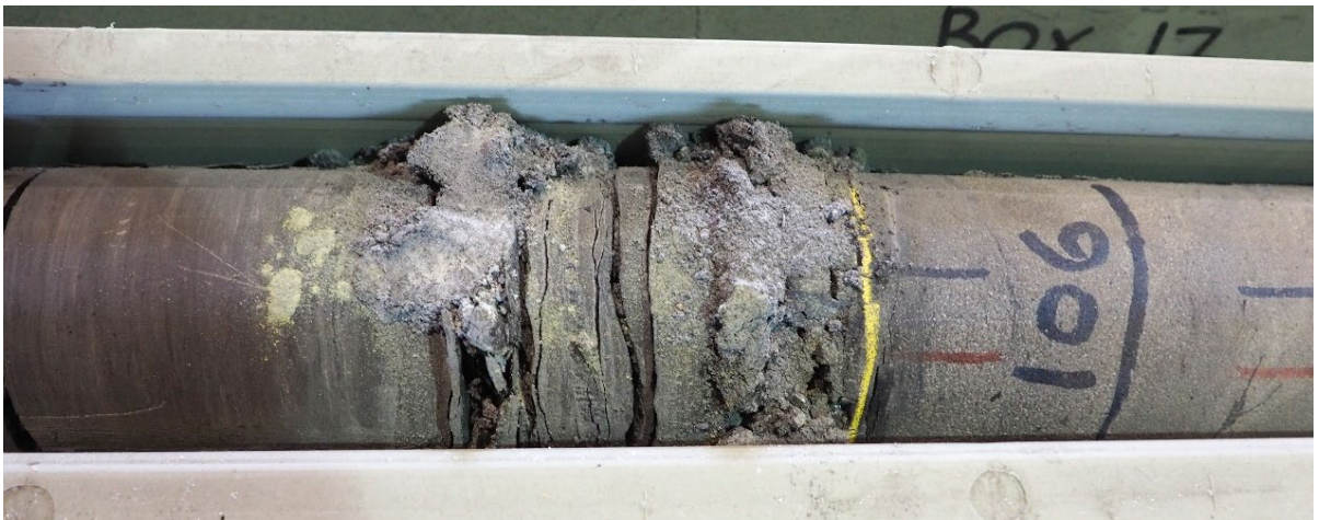
Plate 11: Pyritic zone with sulphate salts in siltstone below Lemington A Seam. Hole 4505C depth 105.9m.
