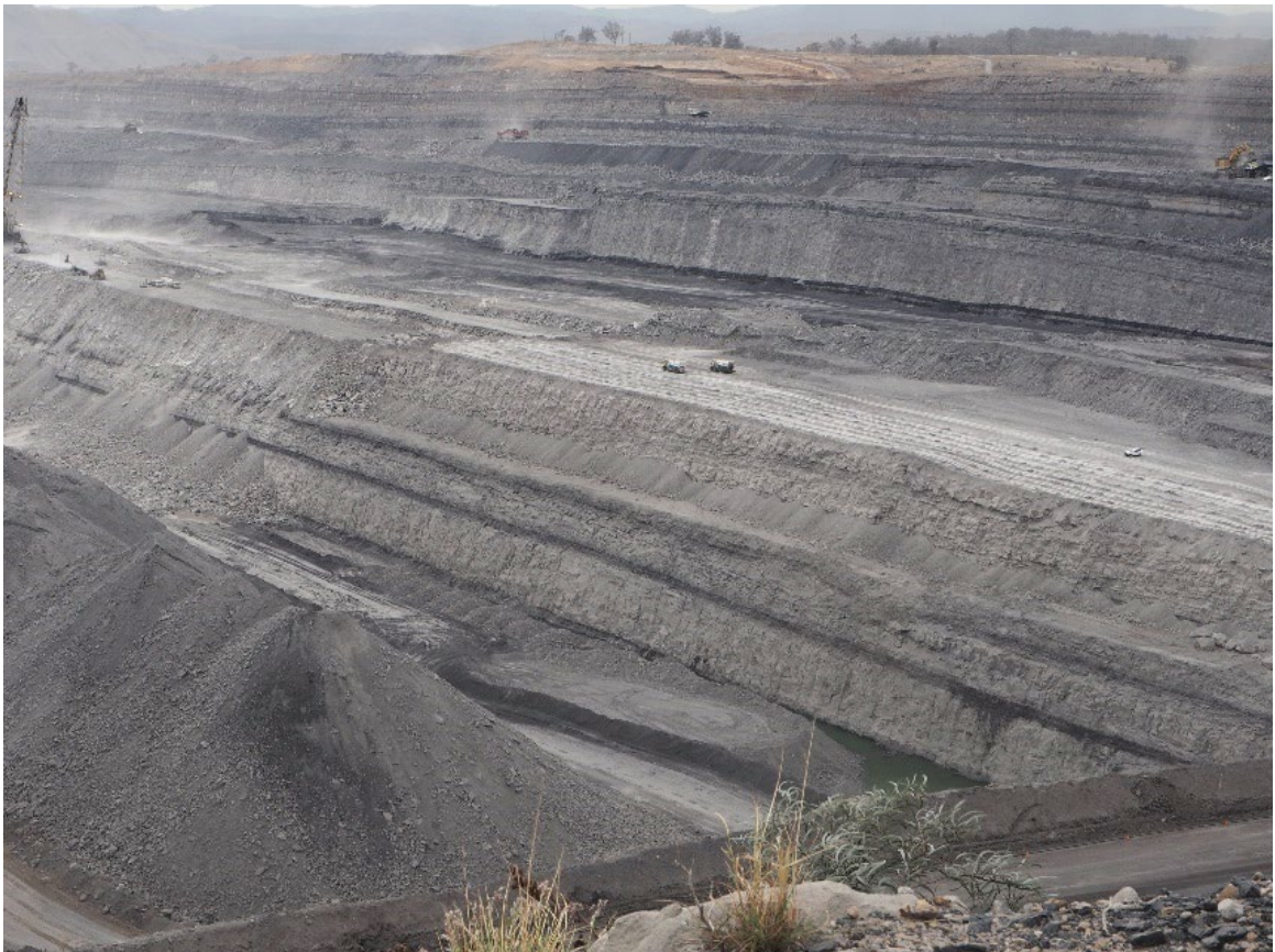
Plate 16: West Pit operations with the majority of the stratigraphy mined exposed down to the base of the Barrett Seam (lower right of photo).
