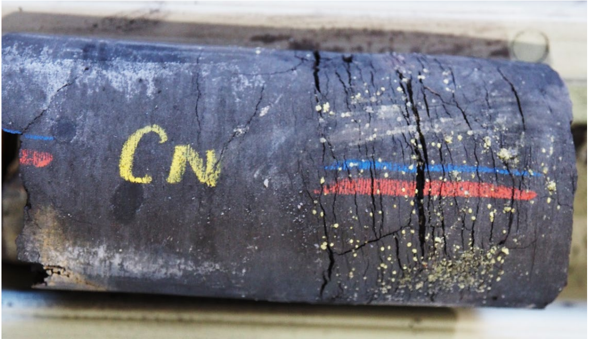
Plate 6: Iron staining and sulphate salts due to the partial oxidation of disseminated pyrite in coal associated with Bayswater Seam Group. 4505C depth 92.8m.
