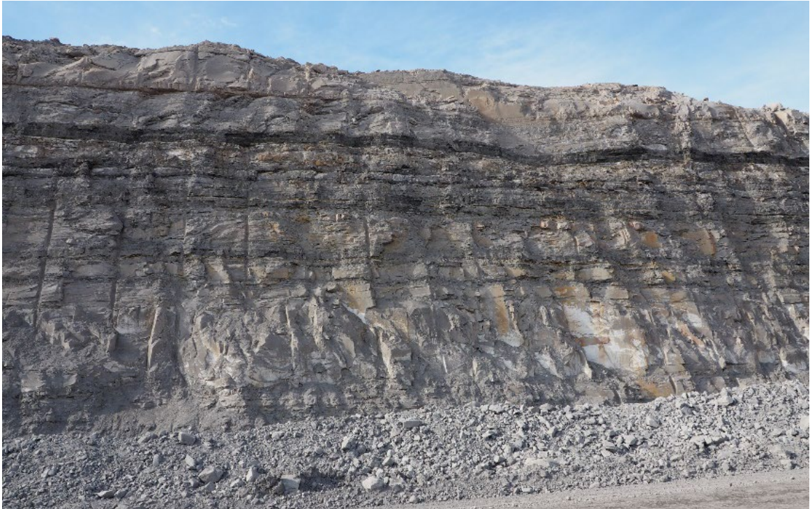
Plate 17: Iron staining and sulphate salts due to the partial oxidation of pyrite associated with the Lemington Seam Group in West Pit.
