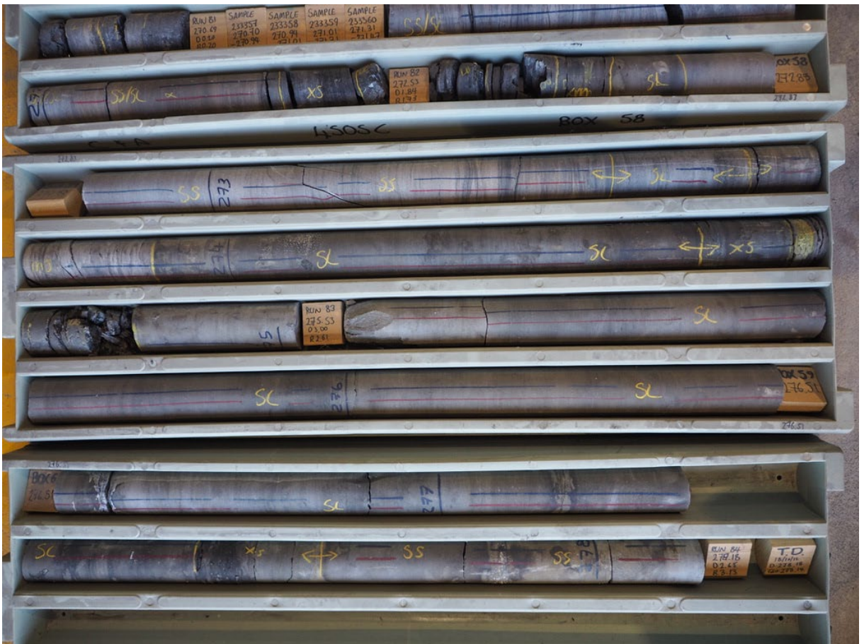
Plate 13: Pyritic zone with yellow tinged sandstone due to sulphate salts with pyrite lenses below the Barrett Seam. Hole 4505C depth 270.49 to 278.18m.
