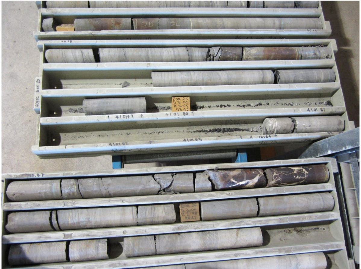
Plate 14: Common siderite lenses with calcitic veining and matrix. Hole 4095C depth 89-97m.
