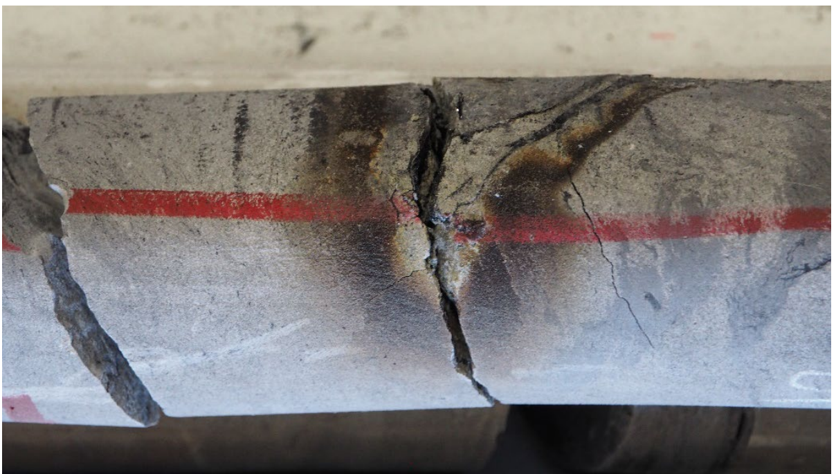
Plate 5: Iron staining due to the partial oxidation of pyrite associated with carbonaceous wisps in sandstone. Hole G3 depth 77.5m.
