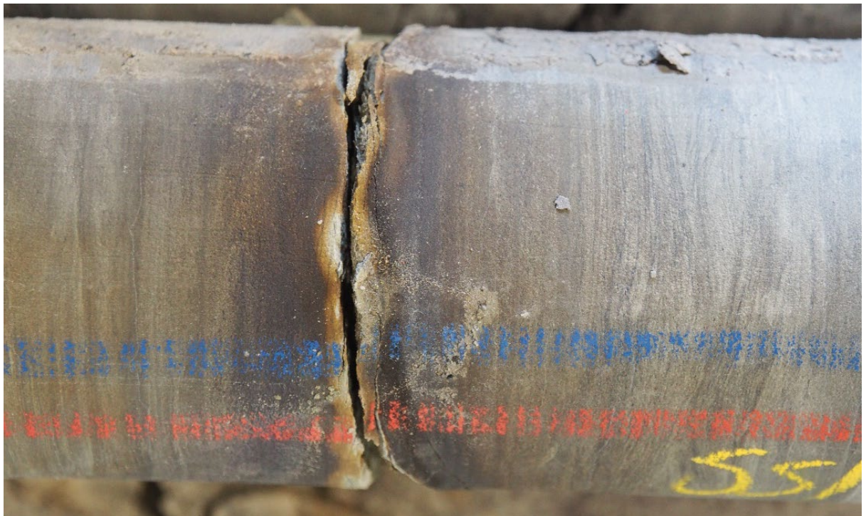
Plate 1: Iron staining and sulphate salts due to the partial oxidation of a pyrite coating on sandstone bedding plane. Hole 4505C depth 59.35m.
