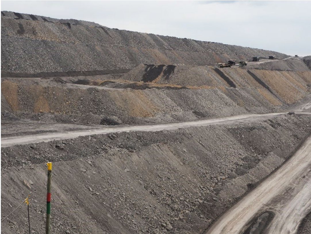
Plate 22: End tipped overburden / interburden dumps within the West Pit.
