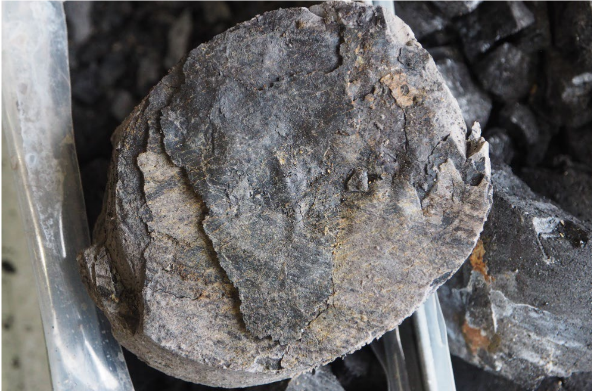
Plate 2: Iron staining and sulphate salts due to the partial oxidation of pyrite on bedding plane of carbonaceous partings within Piercefield Seam Group. Hole GHD23 depth 44.8m
