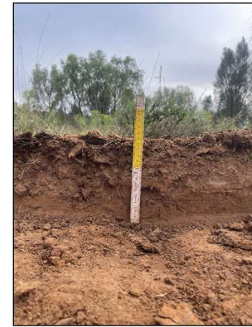
Figure 6: Completed depth at grader scrape 6 (17cm)
