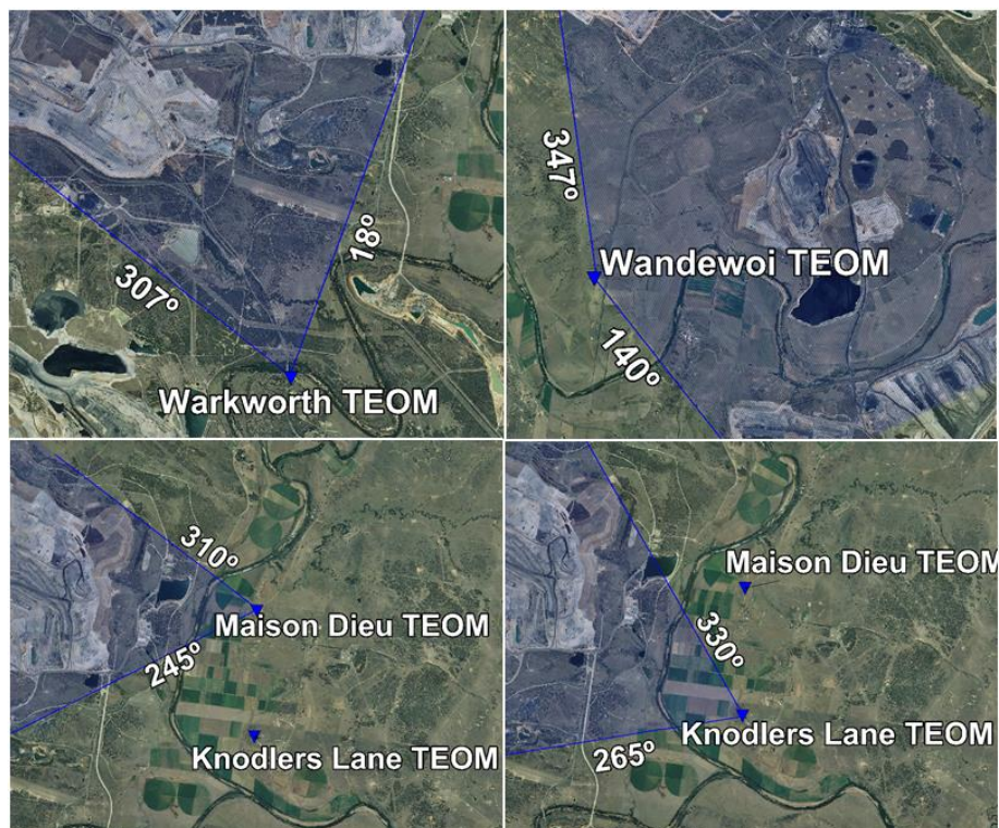
Figure 2: Stage 2 air quality alarms – wind arcs from 'mine to monitor'
