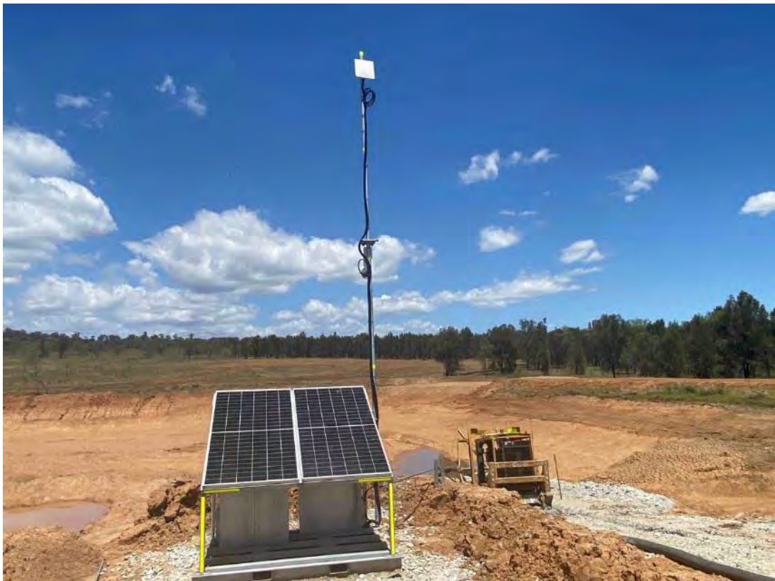
Plate 38 – Example of telemetry water level sensors installed at high risk dams
