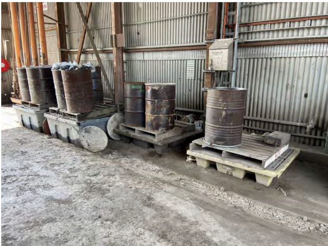
Plate 10 – Portable bunding utilised for barrels and other containers during inspection
