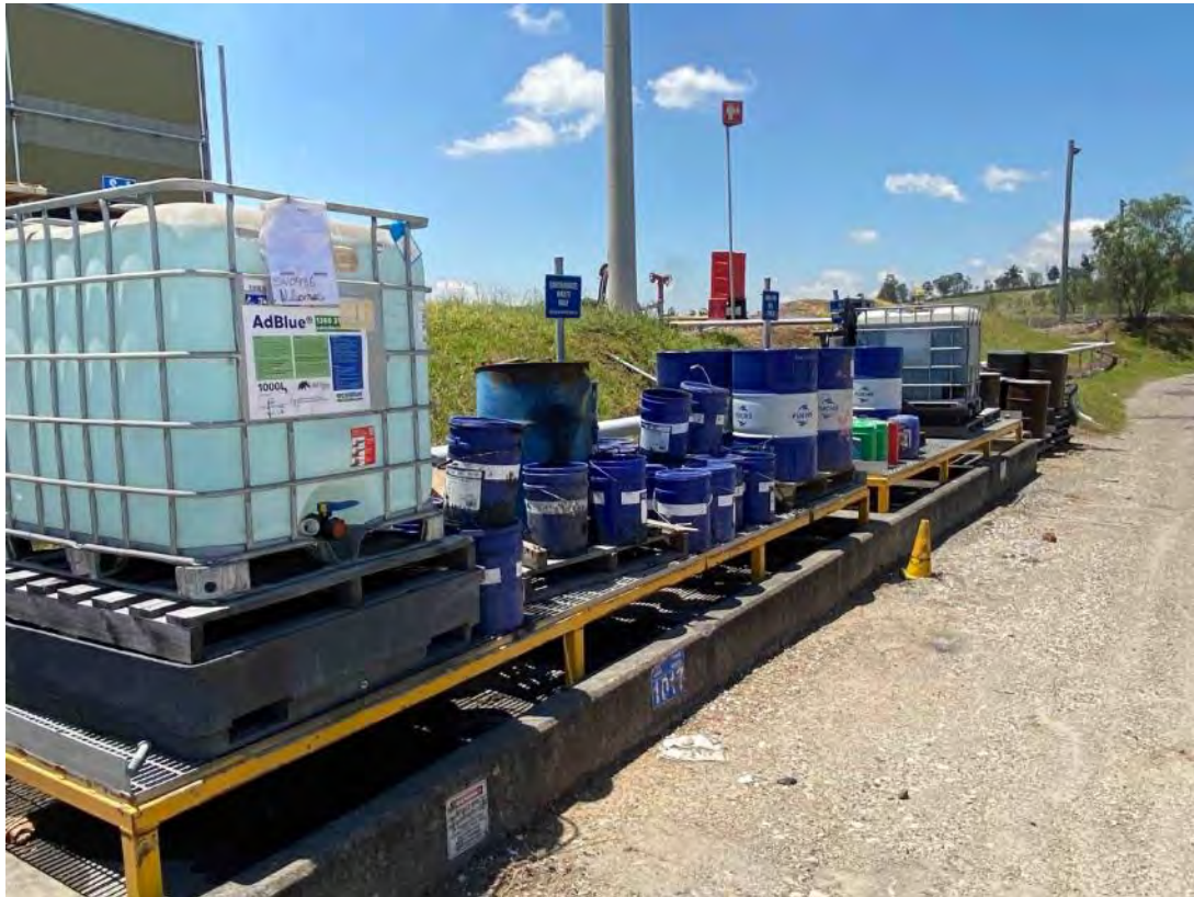
Plate 19 – Suggested lids or cover be placed over uncovered waste containers to limit oily water generation
