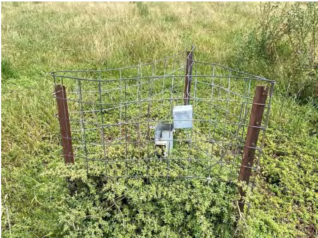
Plate 54 – Groundwater monitoring point with livestock protection structure
