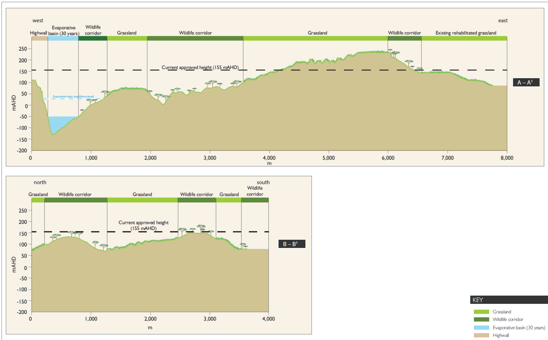
Figure 2: Indicative Final Rehabilitated Landform Cross-Sections
